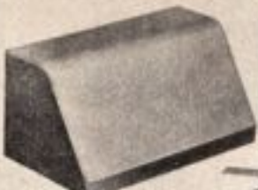
A UNIVERSAL SLOPING PANEL CABINETS—Detachable back-bottom is one piece. Accommodates miniature aluminum chassis. Height 3 3/8", depth 4 1/4". Grey hammertone finish, steel or aluminum.
